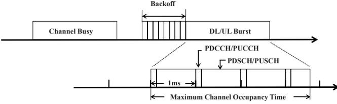
Fig. 1. An illustration of an ID-CSMA data transmission.
