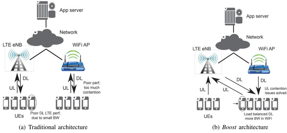
Fig. 2. *Boost* alleviates WiFi network congestion by diverting UL traffic to the LTE network. Moreover, it alleviates LTE DL congestion by moving DL traffic to the WiFi network with large bandwidth.
