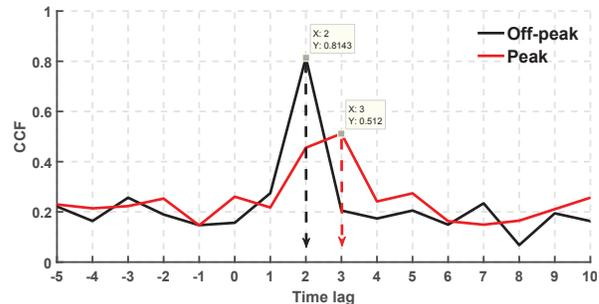
Fig. 2. The CCF between traffic flows measured at traffic detector stations 6 and 3 during two different time periods.
