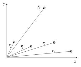
Fig. 4. Localization using time-difference-of-arrival measurements.
