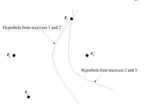
Fig. 6. Intersecting hyperbolas from three receivers.
