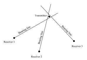
Fig. 5. In the presence of noise, bearing lines from three receivers will not interact at the same point.
