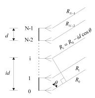
Fig. 2. An antenna array with N antenna elements.
