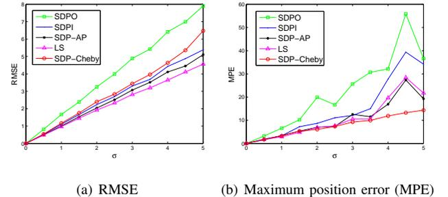
Fig. 3. Localization performance comparison of SDP-Cheby, SDPO, SDPI, SDP-AP and LS under Gaussian distributed measurement errors when the target is inside the convex hull of the sensors. The error bound is  $\gamma = 3\sigma$ .
