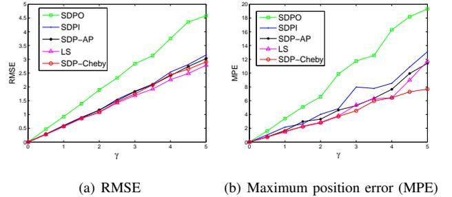
Fig. 2. Localization performance comparison of SDP-Cheby, SDPO, SDPI, SDP-AP and LS under uniformly distributed measurement errors when the target is inside the convex hull of the sensors.
