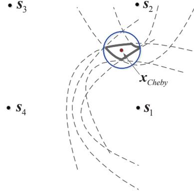
Fig. 1. Chebyshev center of the feasible set for the target.
