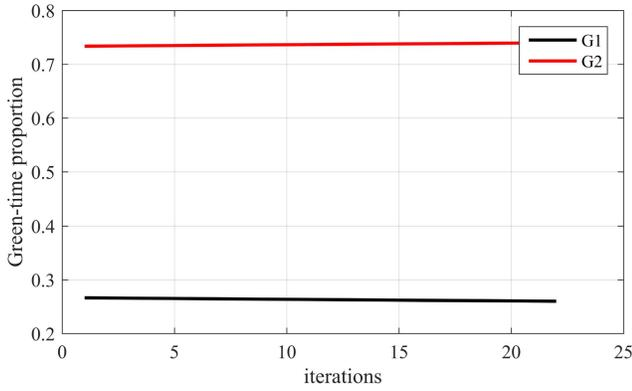
Fig. 10. Time evolution of green-time proportion using novel control policy; the condition of existence of equilibrium is NOT fulfilled.
