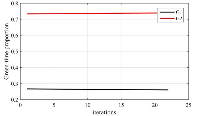
Fig. 9. Time evolution of green-time proportion using novel control policy; the condition of existence of equilibrium is NOT fulfilled.
