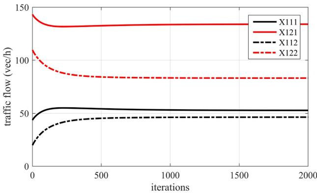
Fig. 11. Time evolution of traffic flow using novel control policy on two-OD two-route network; the condition of existence of equilibrium is fulfilled.
