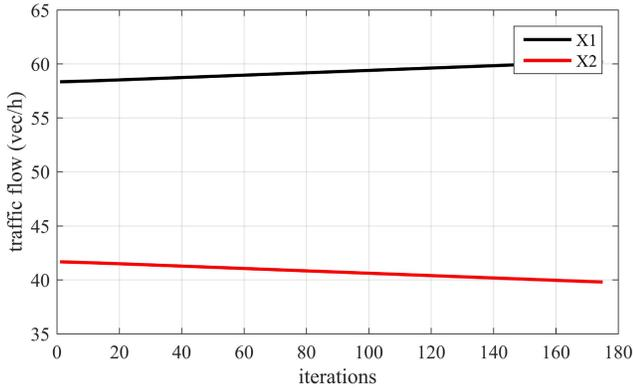
Fig. 6. Time evolution of traffic flow using P0 control policy.
