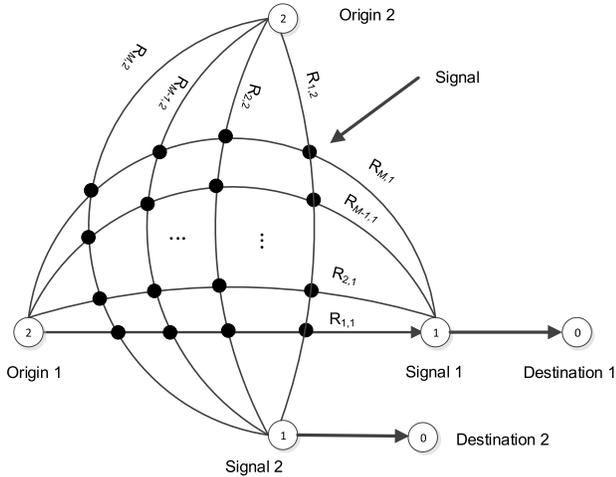
Fig. 2. A signalized network with two OD pairs, where each intersection is equipped with traffic signal.
