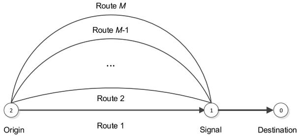
Fig. 1. A  $M$  route signalized network proposed by Smith. Only one OD pair was considered.
