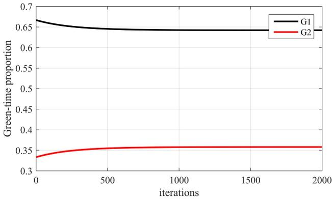
Fig. 5. Time evolution of green-time proportion using novel control policy.
