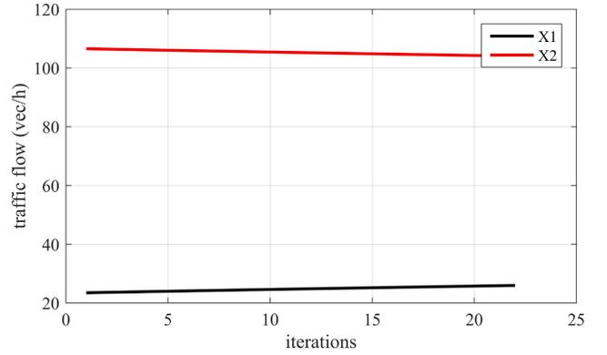
Fig. 8. Time evolution of traffic flow using novel control policy; the condition of existence of equilibrium is NOT fulfilled.
