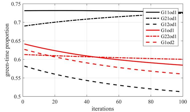
Fig. 14. Time evolution of green-time proportion using novel control policy on two-OD two-route network; the condition of existence of equilibrium is NOT fulfilled.
