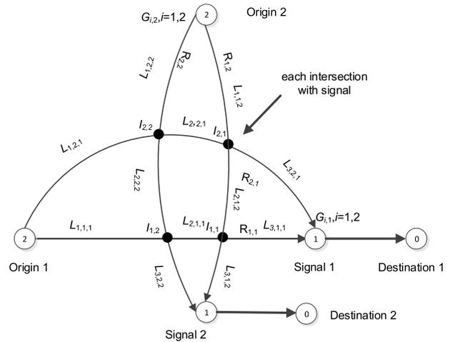
Fig. 3. A signalized network with two OD pairs with two routes each. There is traffic signal at each intersection.
