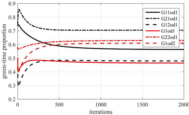
Fig. 12. Time evolution of green-time proportion using novel control policy on two-OD two-route network; the condition of existence of equilibrium is fulfilled.
