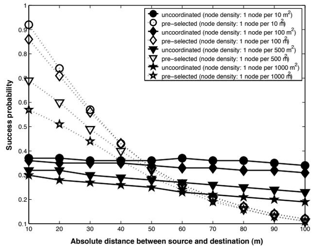
Fig. 4. Success probability vs. source-destination distance for fixed transmission power (set for transmission success probability 0.5 at distance 30m).
