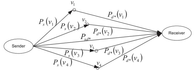
Fig. 1. The system model and notation of link quality parameters.
