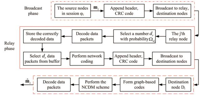
Fig. 2. The data delivery processing procedure.
