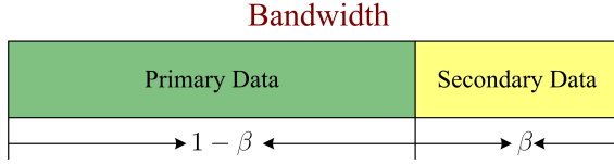
Fig. 2. Bandwidth division between primary and secondary systems. The fraction \beta is released to the secondary system, while the remaining 1 - \beta fraction is kept by the primary system for the direct or cooperative data transmission.
